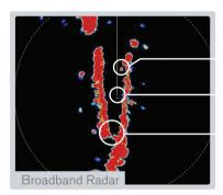
■ Broadband Radar clearly defines this narrow 35-meter channel, showing a small vessel moored near shore and a small footbridge.
