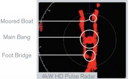
4 kW HD pulse radar can not discriminate the moored vessel from shoreline, "main bang" obscures width of channel.
