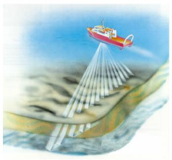
stabilised in both roll and heave (requires a vertical reference unit with analogue outputs) ensuring that the insonified area on the sea floor is accurately positioned.
